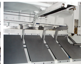
▶ Pneumatic Sheet Support System Optional
