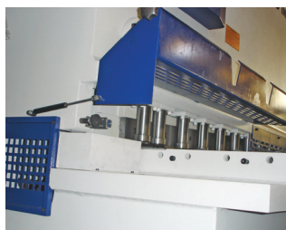
▶ Front Finger Protection Open able 1000 mm
