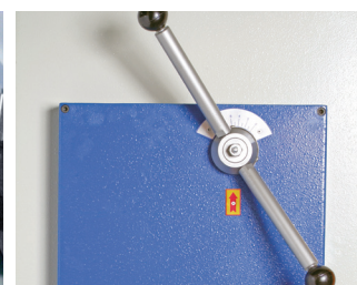
▶ Blade Gap Adjustment system
