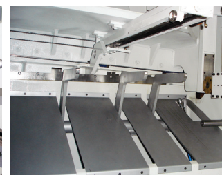
▶ Pneumatic sheet support system Optional
