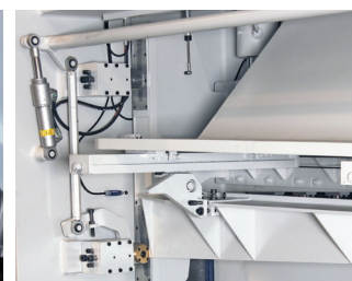
▶ Automatic Blade Gap Adjustment System
