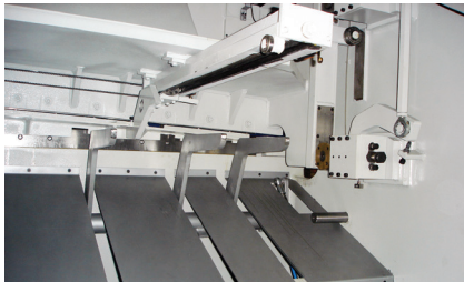
▶ Pneumatic Sheet Support System Optional
