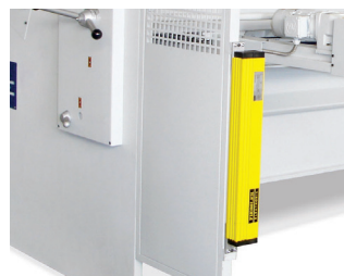
▶ Rear Protection Light Beams
