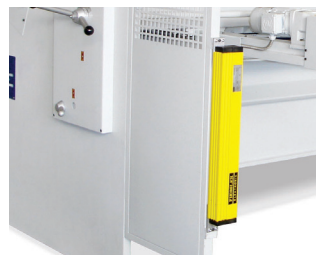
▶ Rear Protection Light Beams
